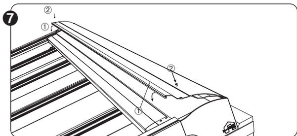
Close the box using the 2 countersunk screws (DIN 966) and a Phillips head screwdriver.
