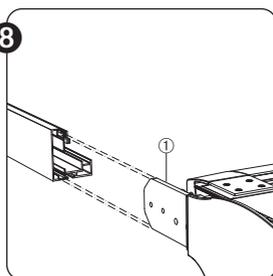
8 Place the open box on the side channels. Insert the pin ① from the box end covers into the dedicated recesses ② in the side channels.
