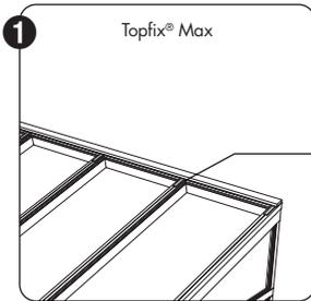
Damping strips (min. 2) should be fitted across the entire width of the box. Cut from damping strip G6020126 (supplied) the same number of pieces as there will be beams under the box. Glue these to the beams on which the box will rest.
