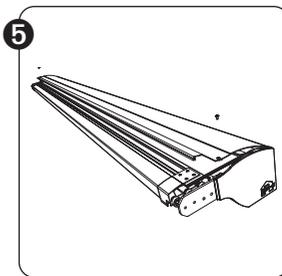
5 The cover of the box should be removed before installing the box on the roof. Do this by removing the 2 countersunk screws (DIN 966) using a Phillips head screwdriver.
