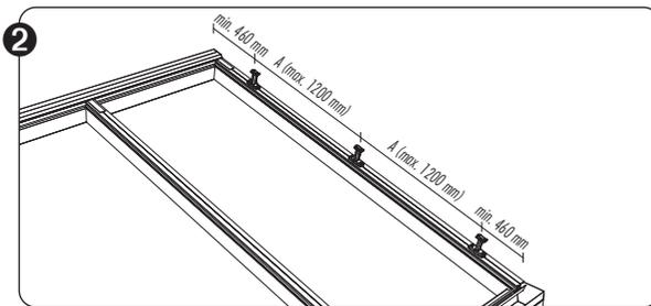
Determine the fastening points for the feet, taking into account the distances shown in the figure. The first foot should be a minimum 460 mm and the last a maximum 500 mm from the outer end of the conservatory/constructions. Locate the other feet every 1,200 mm in between.
