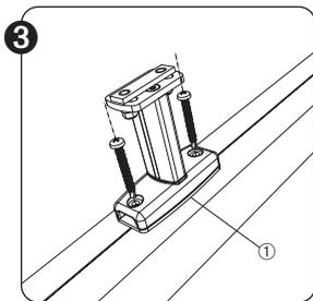
3 Install the supplied assembly feet at their locations. Place a rubber damper ① under each foot.
