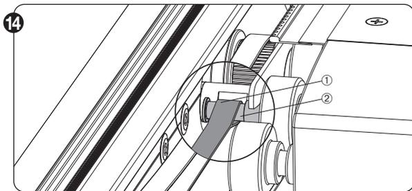
The belt then runs back from the pulley block to the bottom rail. Fit the belt loop ① over the shaft ②.
