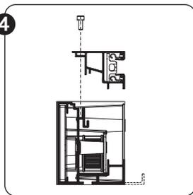
4 Disassemble the side channel. To do so, remove the DIN912 M4x10 screws (Allen key 3).
